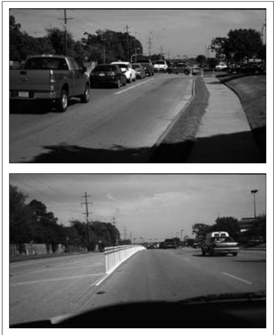
**Figure 2.** Example of the use of flexible pylons as a “retrofit” to limit movements to right-in/right-out. Location: Briarcrest Drive, Bryan, TX
